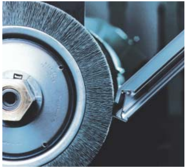
Entgraten von Aluminiumprofilen. Deburring of aluminium profiles.
