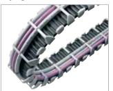
Where more of space is needed, the takeup capacity can be doubled by laying the cables on both sides. In this case every second side-part is simply attached the other way round.
